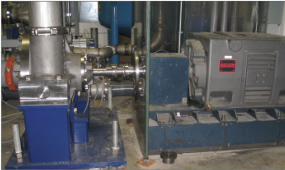
Figure 5 - SSD-1000 HPP with motor and test
